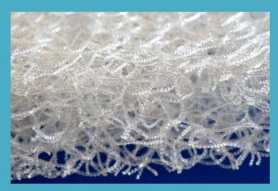
**Techniques:** Use transparent compound Polymer, forming structure once by treatment instead of glue, environment friendly ,will not do harm to water.
